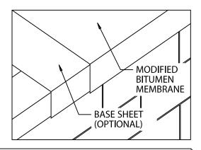
NOTE: Tremco may require a "sacrificial" flashing strip. (Refer to drawing 2A & 2B). Please check with Tremco prior to installation.
